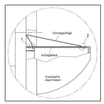
When installing the angled mount, ensure that positions 1 and 2 are correctly located on the base.
