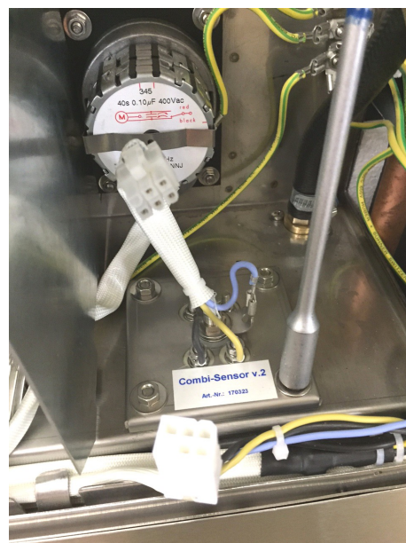
(4x M5) unscrew the nuts
